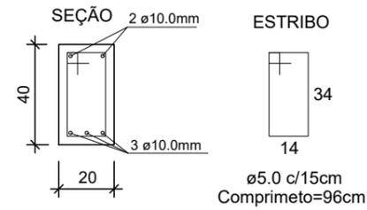
DETALHE VIGA SUPERIOR (V)
